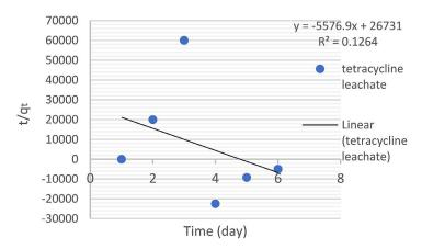
Figure 12. Linear plots of kinetics data of the second order model
