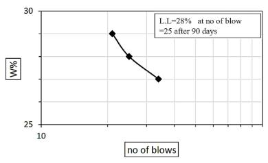
Figure 7. Liquid and plastic limits
