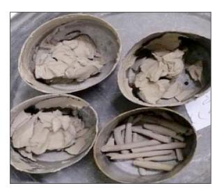
Figure 4. Atterberg limits test
