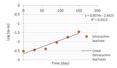
Figure 11. Linear plots of kinetics data of the first order model
